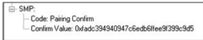
Figure 13 - Initiator Pairing Confirm Example (Wireless Protocol Suite software Main windows, Sodera, Sodera LE Low Energy capture)
