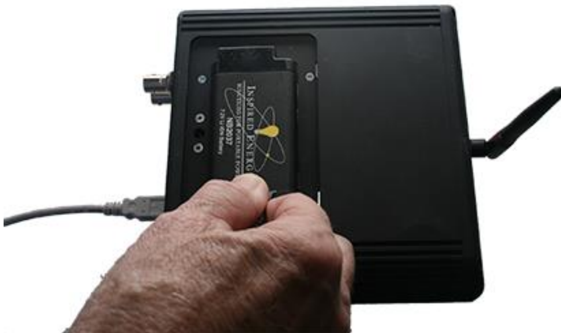
Figure 2.25 - Sodera Battery Removal Using the Tab
