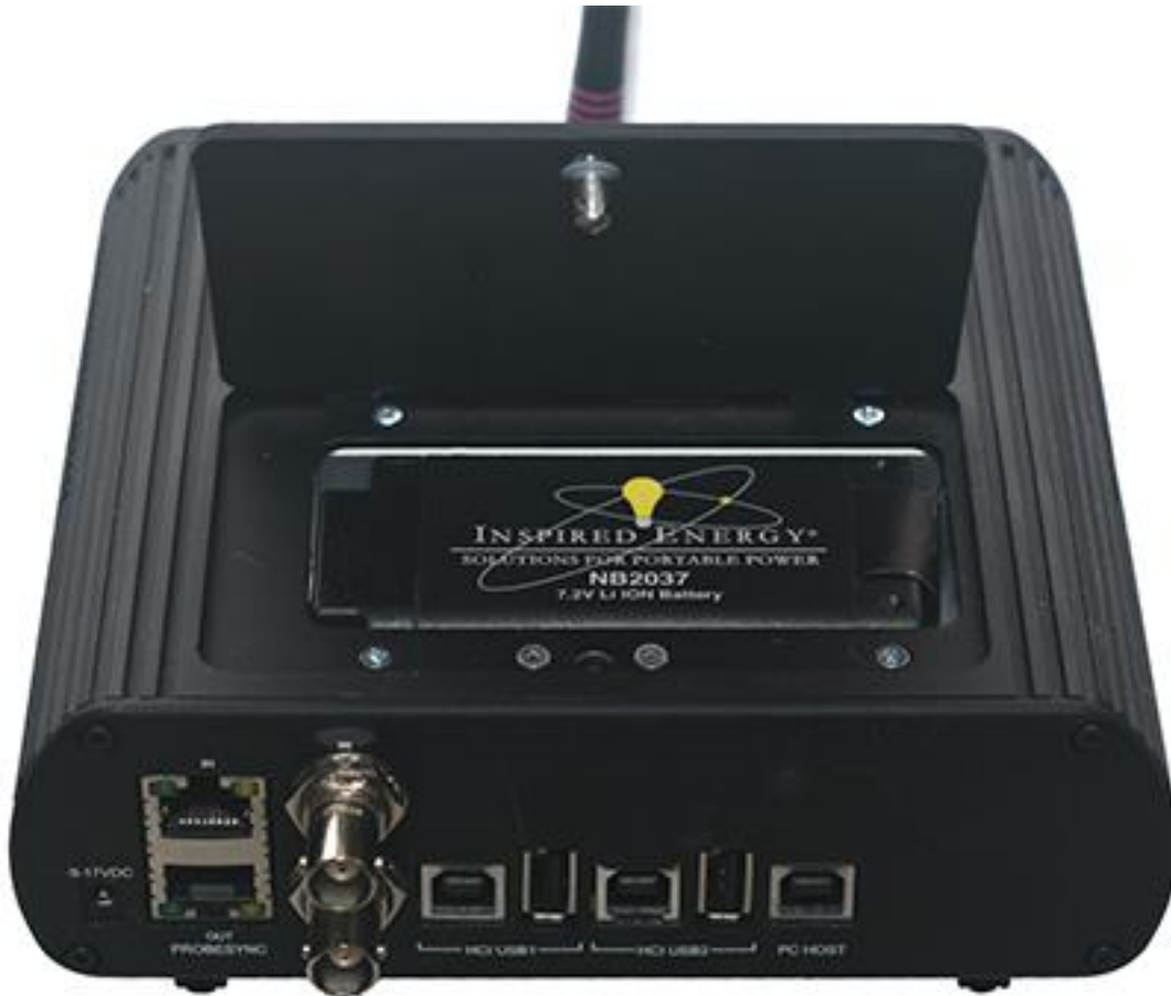
Figure 2.24 - Soderas Battery Compartment with Cover Opened
