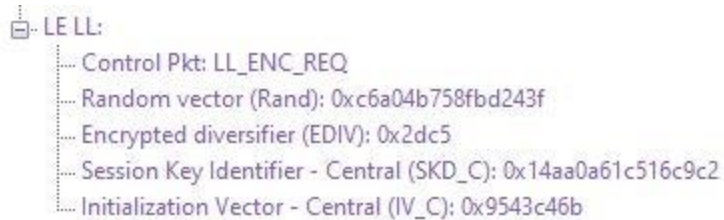
Figure 16 - Encryption Request from Central, Example (Wireless Protocol Suite software Main windows, Soderia, Soderia LE Low Energy capture)
