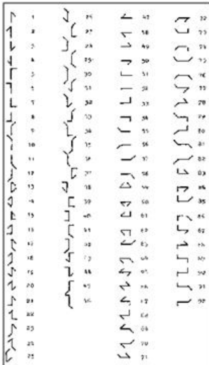
Figure 11 - Chappe's Telegraph Code
