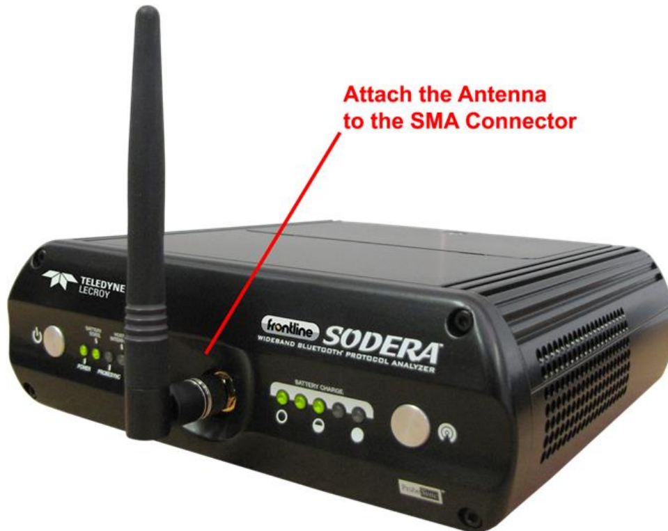
Figure 2.23 - Antenna Attachment Point
