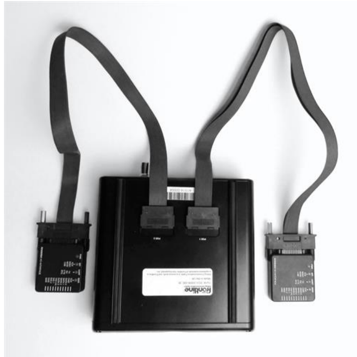
Figure 2.30 - HCI Pods Installed on Sodera
