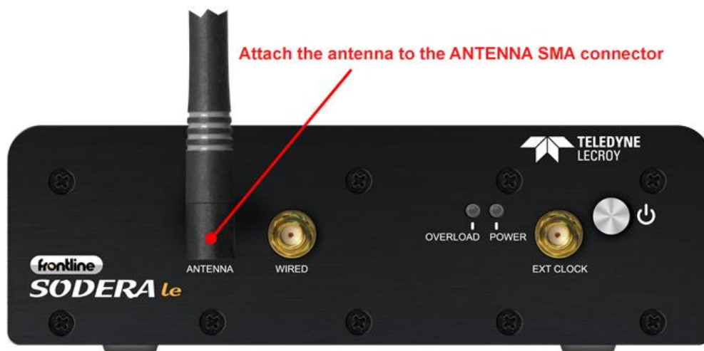
Figure 2.37 - Antenna Attachment Point
