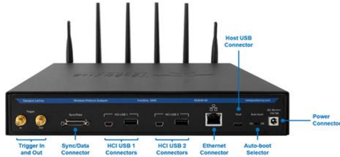
Figure 2.2 - Frontline X500 Rear Panel Connectors
