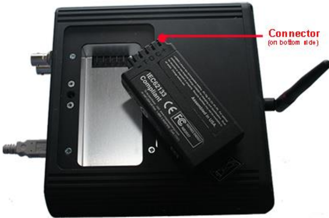
Figure 2.26 - Sodera Battery Connectors, bottom side shown.
