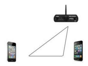
Figure 3 - For Audio A2DP, Position Closer to SINK DUT
