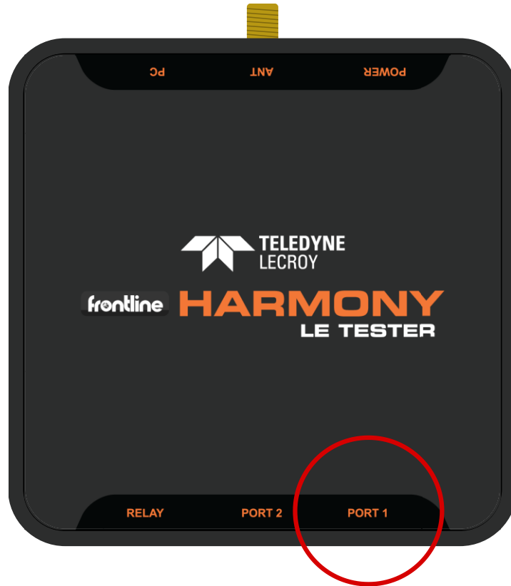
Figure 13 – IUT Port Connections
