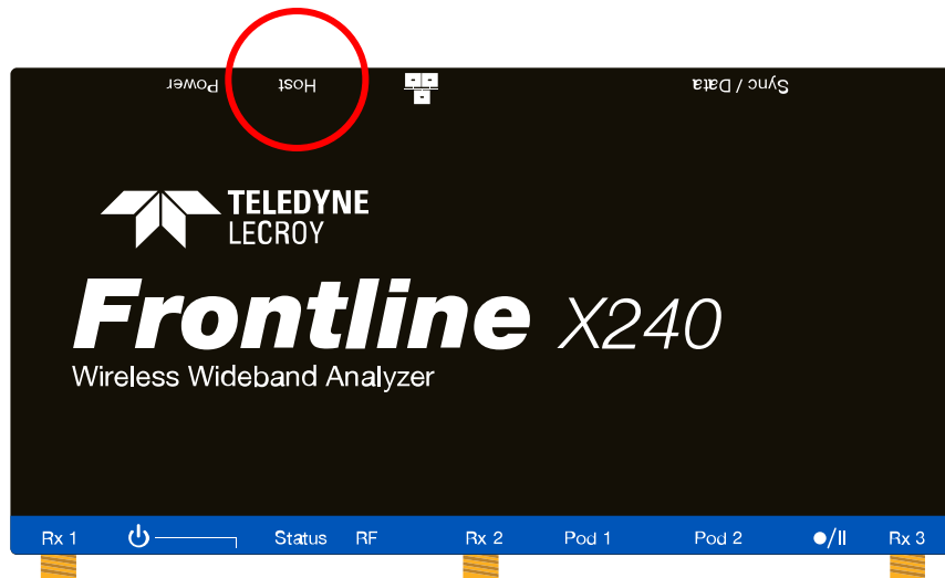
Figure 14 – Soderia and X240 PC Connections
