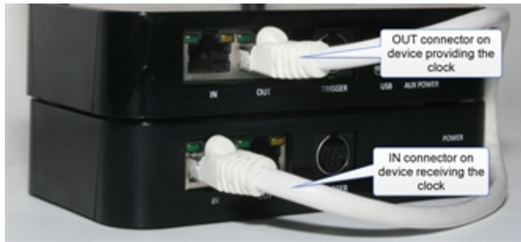
Figure 2.5 - BPA 600 Hardware ProbeSync connection
