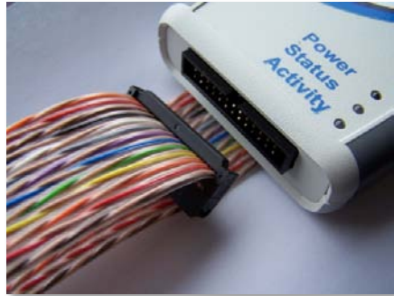
Figure 1: SD/SDIO/SPI/MMC hardware interface with ribbon connector
