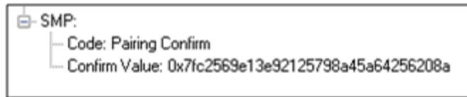
Figure 14 - Responder Pairing Confirm Example (ComProbe Frame Display, BPA 600 low energy capture)
