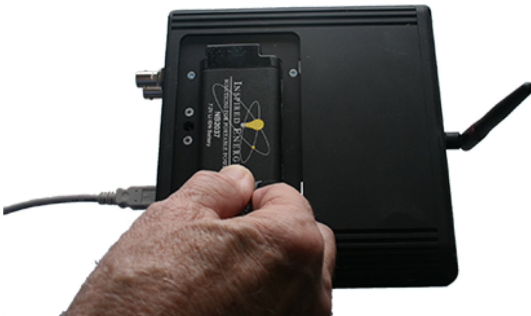
Figure 2.5 - Sodera Battery Removal Using the Tab
