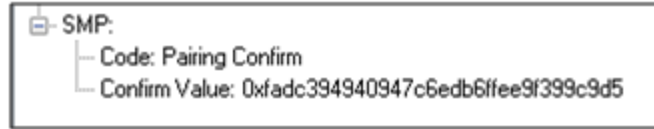
Figure 30 - Initiator Pairing Confirm Example (ComProbe Frame Display, BPA 600 low energy capture)
